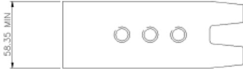
Figure 10 - Plunger dimension limits
