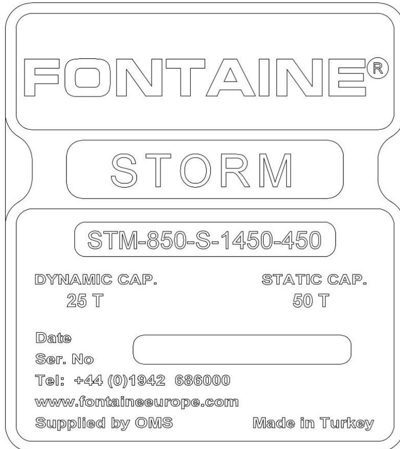
There is a lable on every landing gears that indicates informations about the producer, products,the dynamic and static capacity of landing gears and production date.
